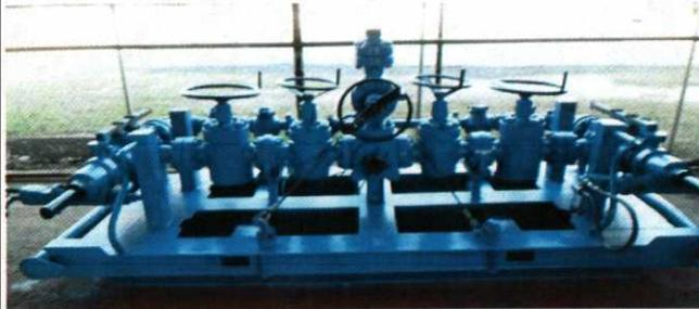
5 Valve Hyd. Choke Manifold
