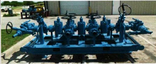
9 Valve Hyd. Choke Manifold
